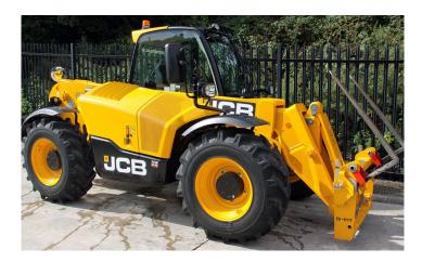
Max lift capacity **3,170kg**Max lift height **7,000mm**Max forward reach **3,700mm**Capacity at maximum reach **1,250kg**Engine power gross **75hp(55kW)**
